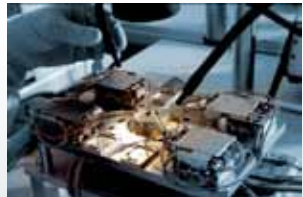
Microprober for conductivity measurements
