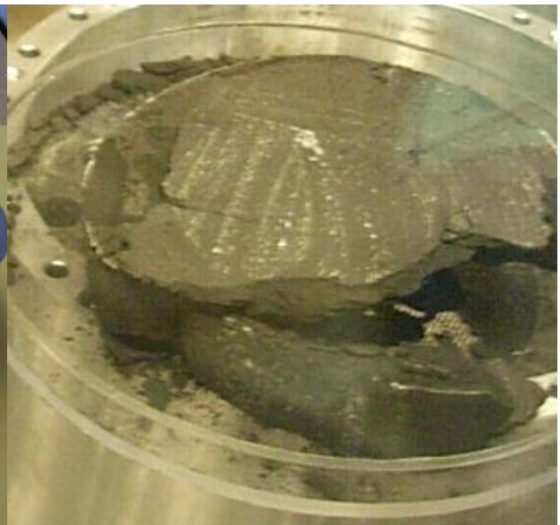
Figure 2: early compacted disk removed from the matrix
