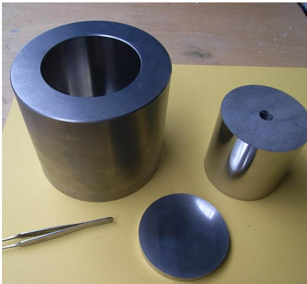
Figure 1: Embossing tool ( \varnothing = 80 \text{ mm} )
