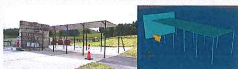
Figure 1. Test facility (left), FLACS geometry (right)
