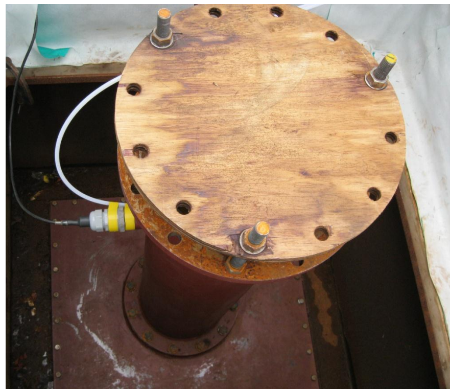
Chimney fitted with hydrogen sensor, manometer and shield block
